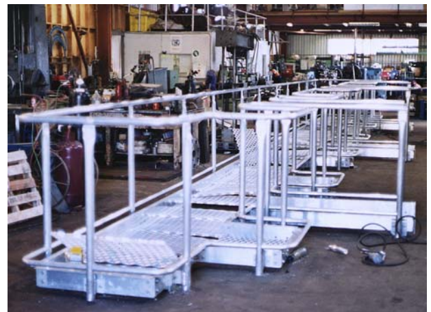
Platform trial assembly in workshop
