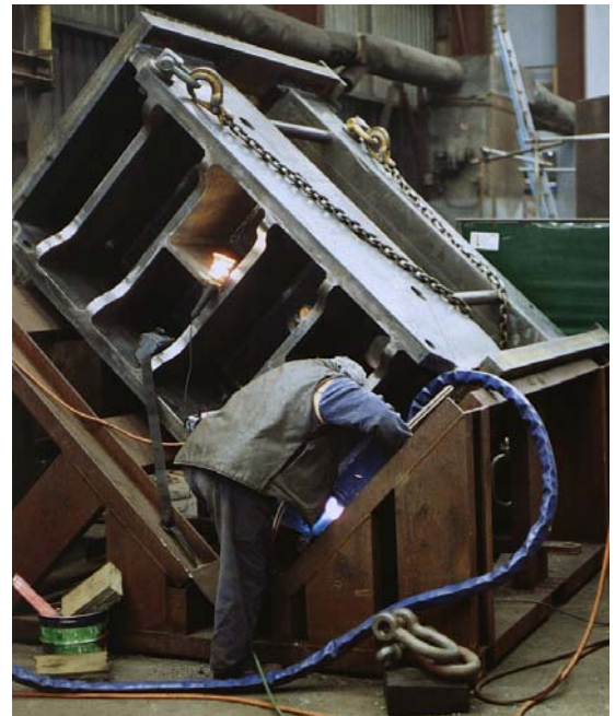
Panel press – assembly welding
